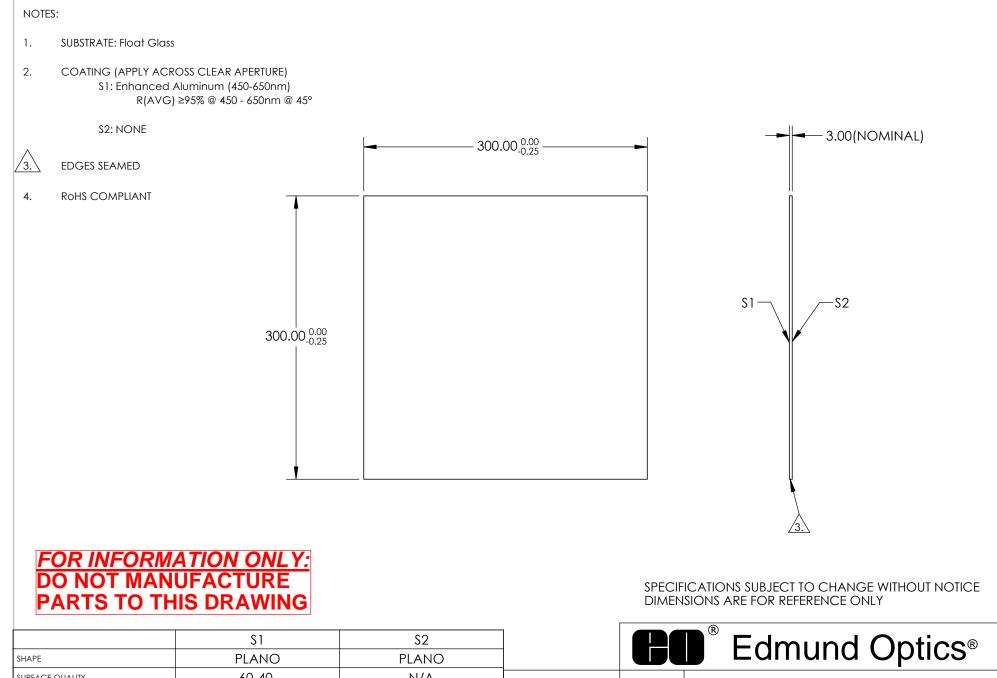
N/A SURFACE QUALITY 60-40 300 x 300mm, Enhanced Aluminum, 4-6λ THIRD ANGLE 4 - 6λ N/A TITLE SURFACE FLATNESS Mirror 270.00 x 270.00 N/A CLEAR APERTURE SHEET DWG NO ALL DIMS IN mm PROTECTED AS NEEDED PROTECTED AS NEEDED 29420 BEVEL 1 OF 1
